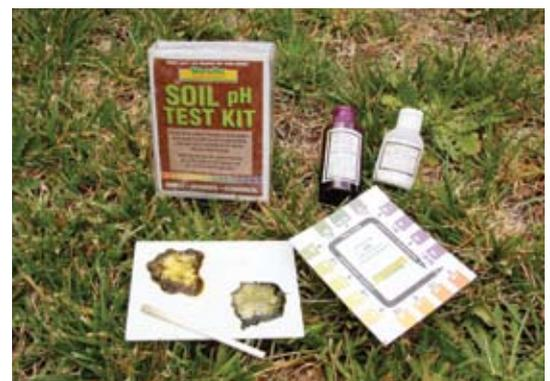
Figure 5: pH field test kit
