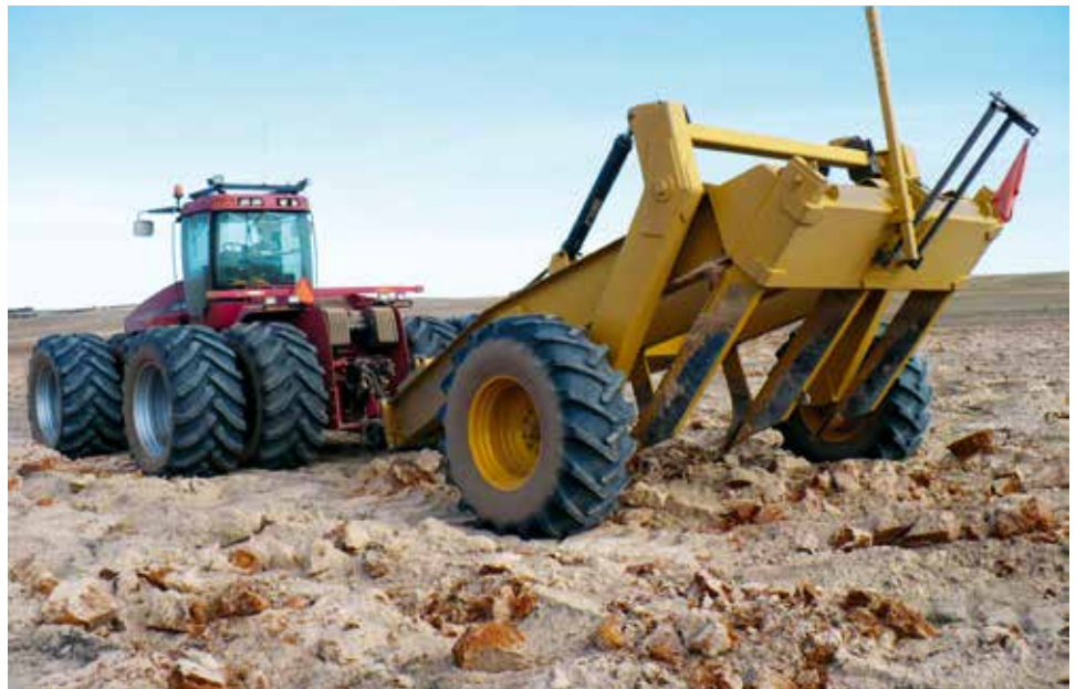
Delving uses specially-designed machines to rip deep into the soil profile and pull up the clay-rich subsoil, incorporating it into the sandy soil.
